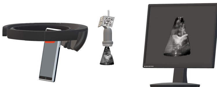
Figure 6. The schematic setup for measuring the latency of displayed US volumes. A slow-motion video captures the US station screen and the rendered US volume.
